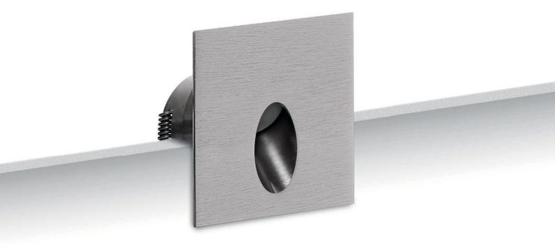
▲ ② ④ C.C. ★ IP44  $\widehat{}$ Quara\_R | Path-marker | powerLED 2 W 630 mA (f)) 52 colour optic type Nickel CRI 80 86402 3000 K 208 lm w 70° 70 42 4000 K 222 lm Ν С 5000 K 253 lm R - G - B - Y on request -89147 99115 99114 84338 ON/OFF 1 - 2 art. 1-10V 1 - 10 art. DALI 1 - 10 art. Outer casing
